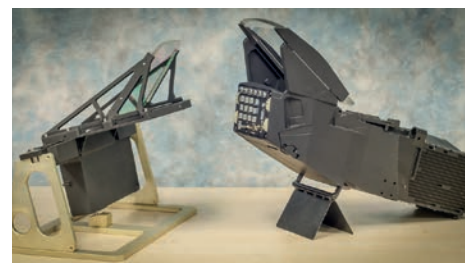
Image courtesy of BAE shows the LiteHUD (left) next to a conventional HUD (right)
